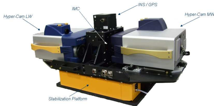
Figure 2: Illustration of the airborne configuration with two Hyper-Cams
