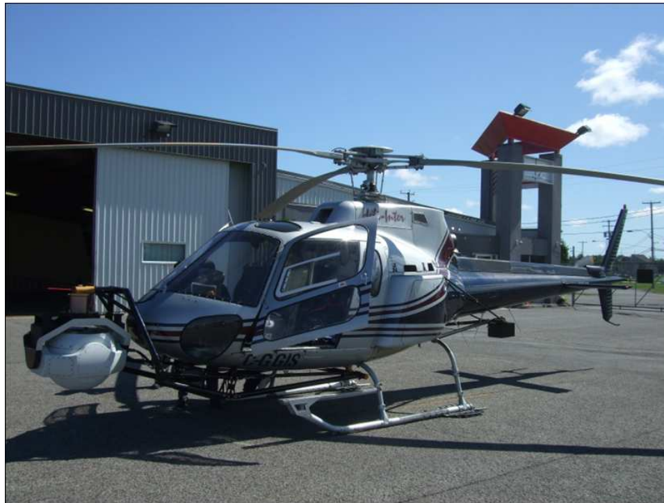
Figure 4: The Telops Hyper-Cam in a PV Labs Look Down Gimbal
